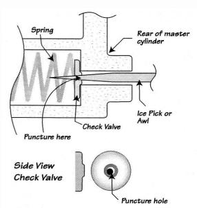
Warning! If not punctured correctly it will cause your disc brakes to drag and overheat causing premature pad wear and possible brake failure.
